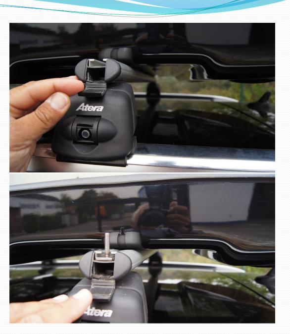
Lift the box and place the T-adapter in each case under the slot
